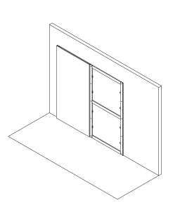
**\_6** Hook the wall panel through the pre-mounted frame supports and the respective ones pre-installed on the panel.
