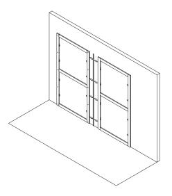
**\_4** Place the alignment band into the proper miling on the frame. Place the second frame mortising it, throught the proper milling, with the first one, already fixed to the wall.
